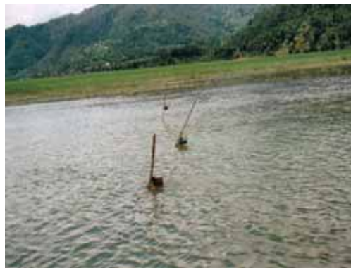
Vertically set drift net into River
