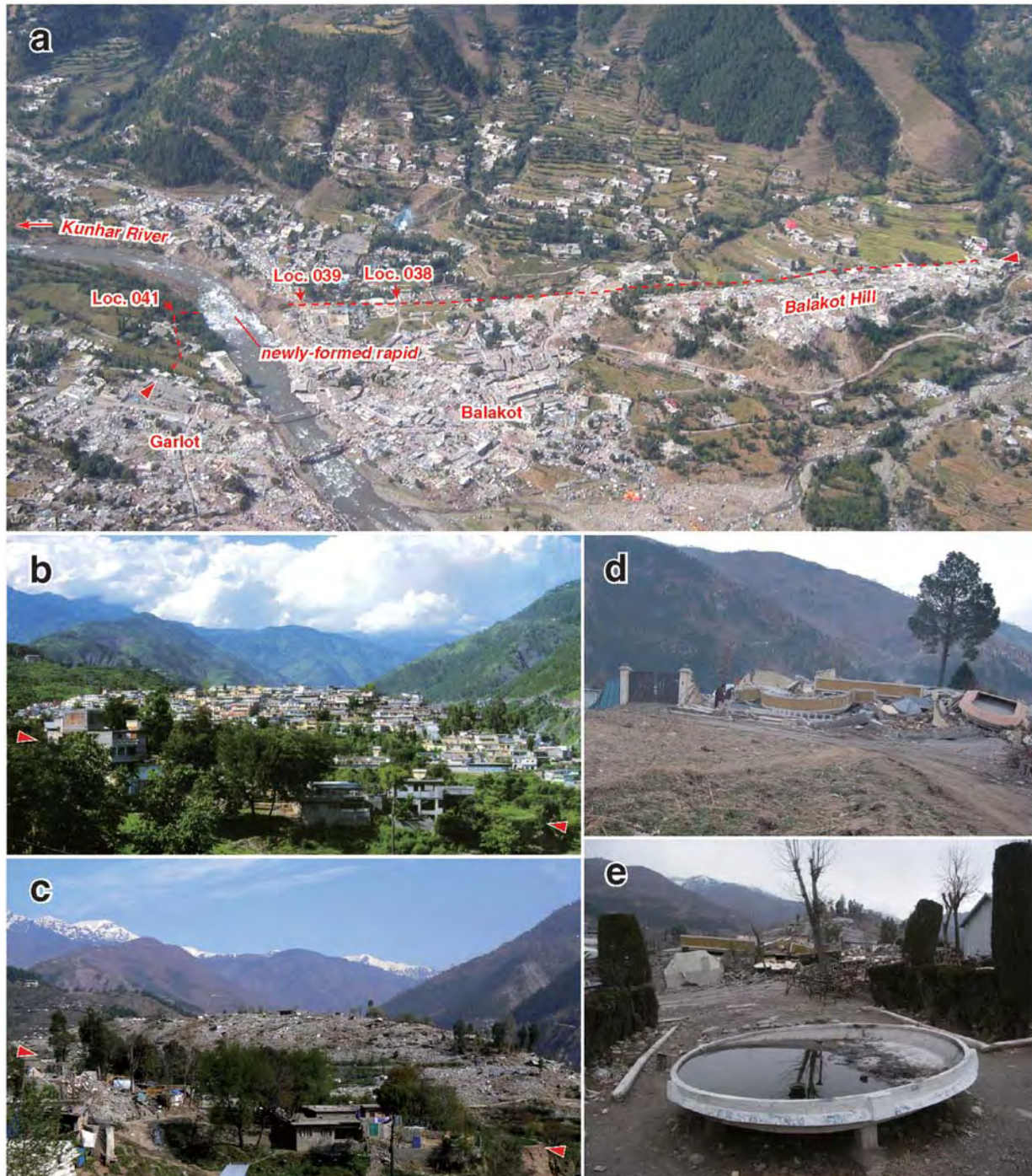
Figure 5. (a) Oblique aerial photograph of Balakot taken one week after the earthquake during the United States helicopter relief mission. View west. The surface rupture trace is shown by a dashed red line, with red arrows indicating selected numbered localities. Note that structural damage is concentrated on the hanging-wall side (bottom side) of the thrust surface rupture. Photograph is courtesy of Wiley Thompson. (b) and (c) Balakot Hill (Old Balakot) before (b) and after (c) the earthquake. Looking northeast. Balakot Hill is interpreted as a tilted or warped remnant of a fluvial terrace surface, a causative fault presumably running along the southwestern margin of the hill (indicated by red arrows). The 2005 surface rupture appeared along this active fault trace, leaving incredible devastation on the hill. The preearthquake photograph is on the courtesy of Aamir Rashid. (d) Westward tilting of the base of the destroyed yellow-painted house (location 038) just southeast of Balakot Hill. The vertical separation is measured to be \sim 2.65 m here. Note that a tree on the background is also tilted. (e) Westward tilting is most clearly demonstrated by a small fountain basin at a school southeast of location 038. Looking northwest. The yellow-painted house and Balakot Hill are visible on the background.
