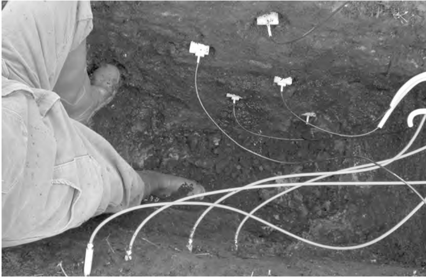
Fig. 9 – TDR probes (upper) and temperature sensors (lower) soon after their establishment.
