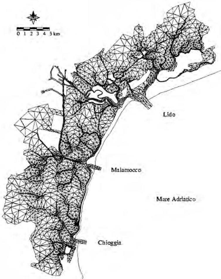
Fig. 1 - Finite element grid of the Venice lagoon adopted by the hydrodynamical model.
