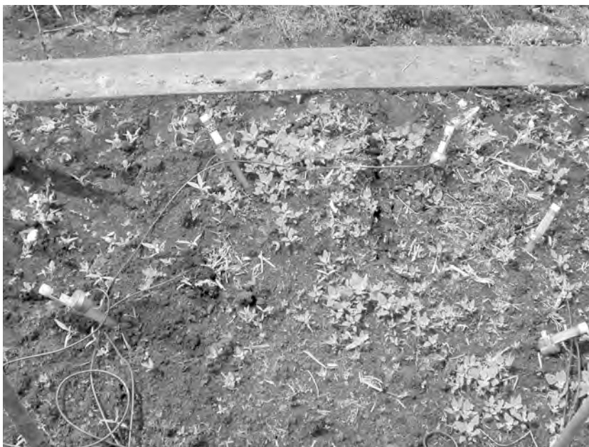
Fig. 8 – Tensiometer location within a test site.
