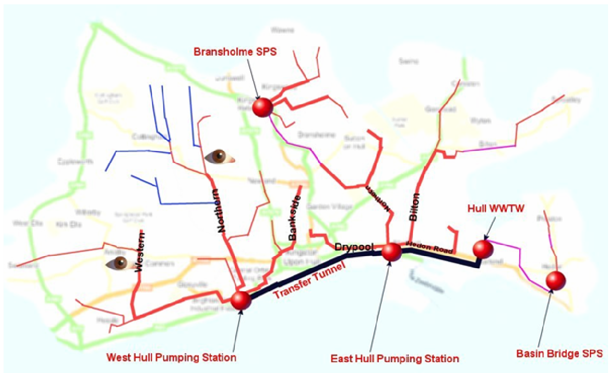
Figure 6.3 Present day drainage system (source Yorkshire Water).
