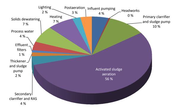
Figure 2. Energy breakdown of wastewater treatment plant with activated-sludge treatment (Based on Tchobanoglous, et al., 2004)
