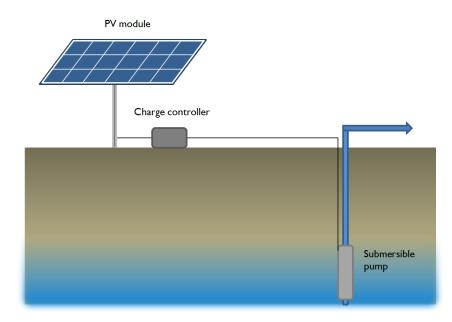
Figure 8. PV module system components in water pumping
