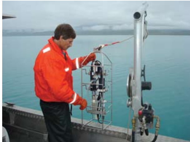
Figure 4. The CTD ready to be deployed at an oceanographic station.
