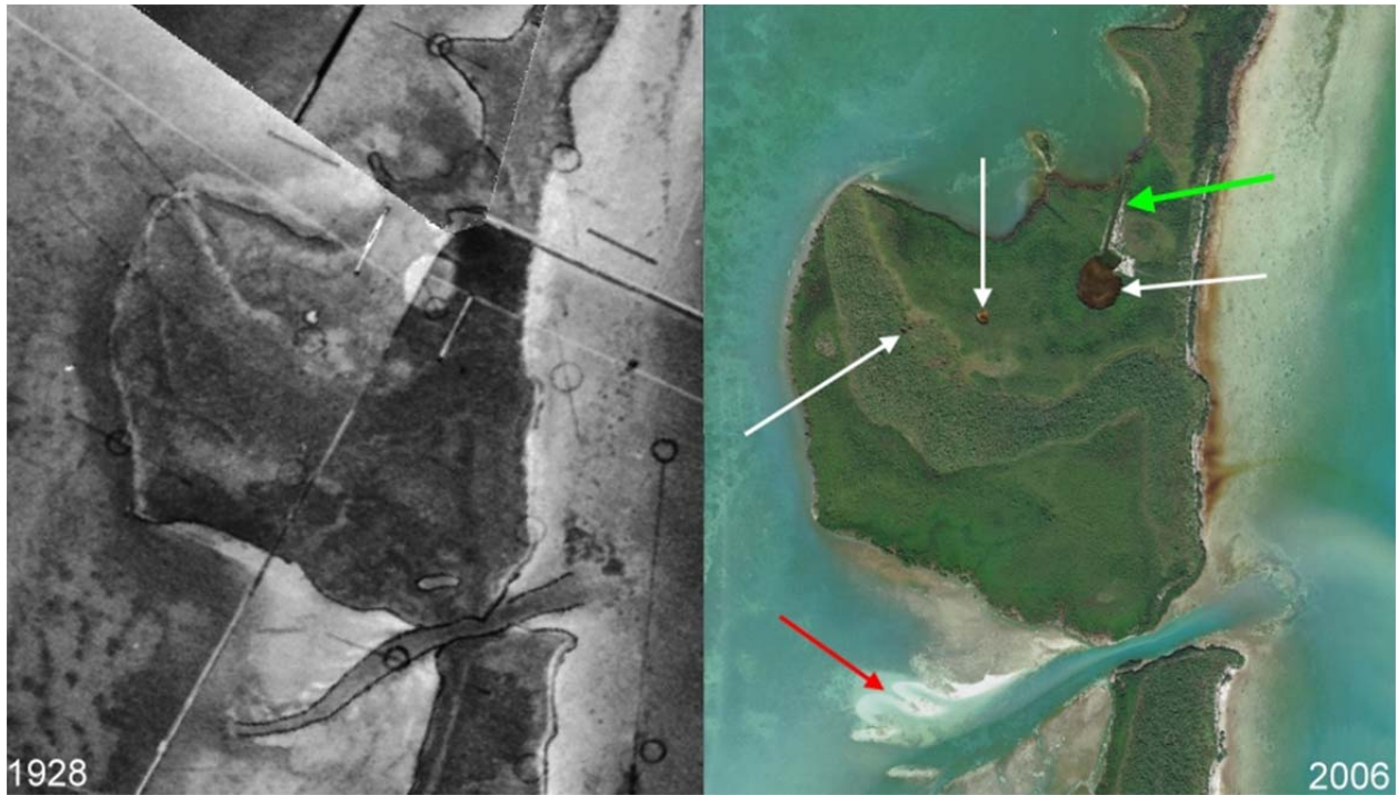
Figure 41. Aerial photos of Sands Key showing dolines formed in Key Largo Limestone. The photomosaic on left is from the first aerial coastline survey by Coast and Geodetic Survey in 1928. It includes interpretative marks (black outlines and alignment circles) from the originals. The white arrows on the right image (2006, FLADOT) show a large (~160 m) and two smaller dolines (42 and 15 m). The sinuous band across the island is an elevated rock feature with hardwood hammock vegetation with numerous smaller dolines. The green arrow is a dredged channel dug that connects to the large doline. The red arrow points to an area of significant erosion in the tidal channel margin since 1928, which has changed the flood delta morphology; above that, there appears to be more mangroves on the south shore.
