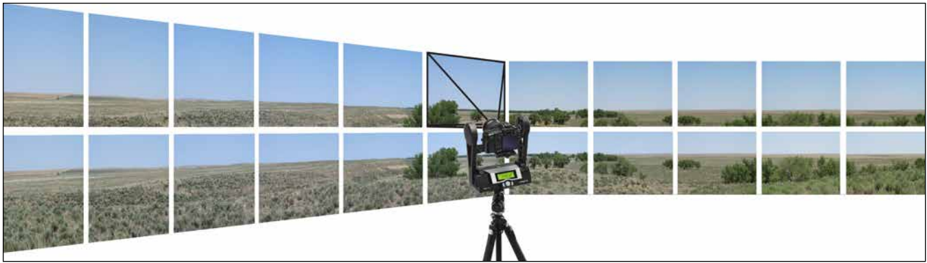
Figure 4.1.2-2. The GigaPan system takes a series of images that were stitched together using software to create a single panoramic image.
