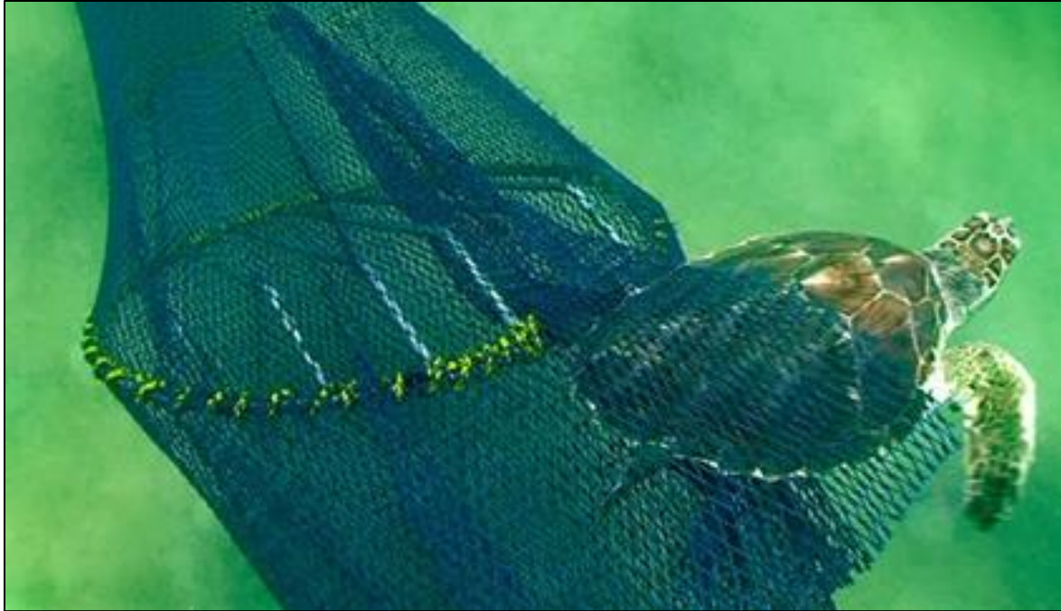
Figure 65. A sea turtle escaping a fishing net through a TED (NMFS photo). Shrimp and other targeted species are small enough to pass through the metal bars, but turtles are stopped and can swim out through a loose mesh opening.
