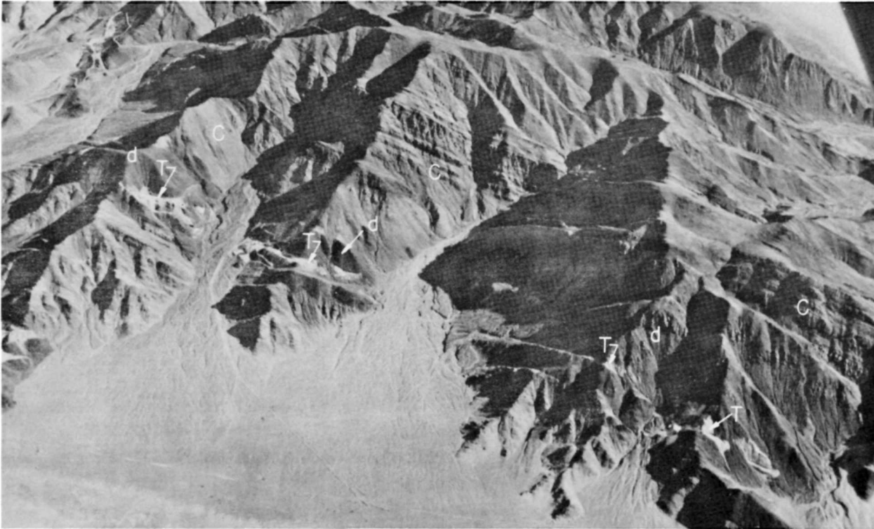
Photo 23. Saratoga talc mine in the Saratoga Hills as viewed from the west on January 14, 1976. This is the southernmost talc mine in Death Valley National Monument and is in San Bernardino County. Most of the mine workings are underground, although there are some surface cuts. Talc bodies (T) and adjacent silicated zones are completely enclosed in diabase (d) which intrudes the Crystal Spring Formation (C).
