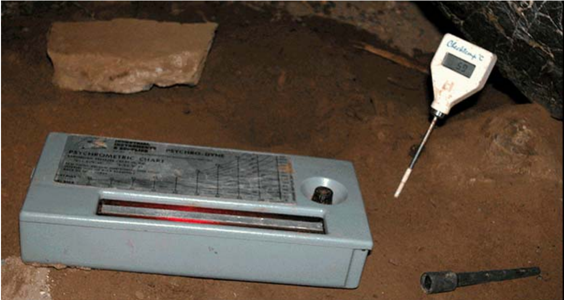
Figure 34. Gray box is wet-bulb/dry-bulb humidity meter, used to measure humidity and air temperature. White probe is used to measure soil temperature at 2 cm depth.
