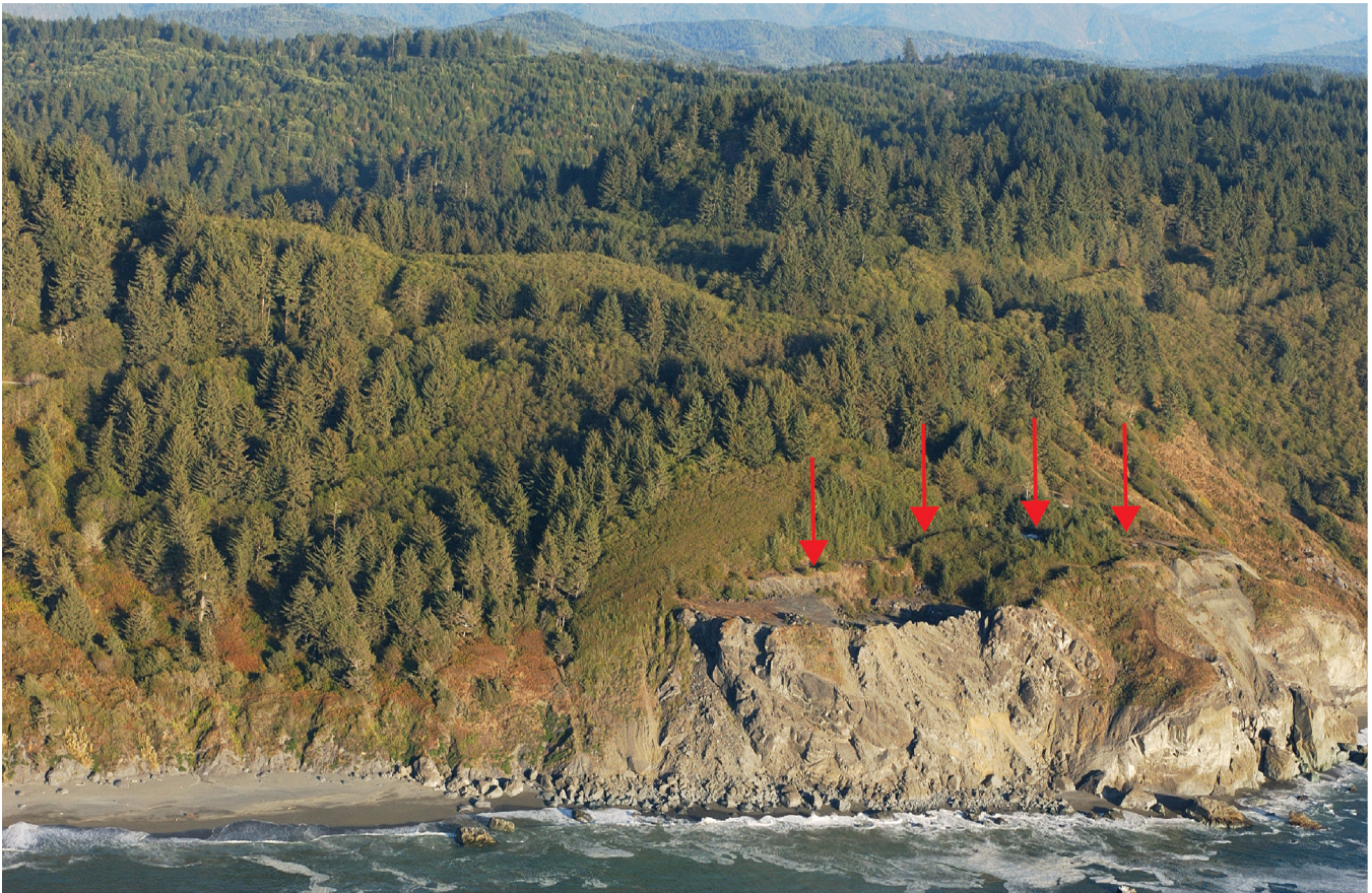
Figure 18. Photograph of Franciscan Complex and resulting landscape. The landslide-prone Franciscan Complex makes up much of the parks' landscape. South of the mouth of the Klamath River (near Flint Rock Head), the mélange unit of Crescent City area (KJfmc) yields hummocky terrain indicative of landslides. The red arrows point to a scarp at the top of a landslide deposit. Photograph (Image 7393, taken 13 October 2002) by California Coastal Records Project. Copyright © 2002–2021 Kenneth & Gabrielle Adelman, California Coastal Records Project, www.californiacoastline.org , used by permission.
