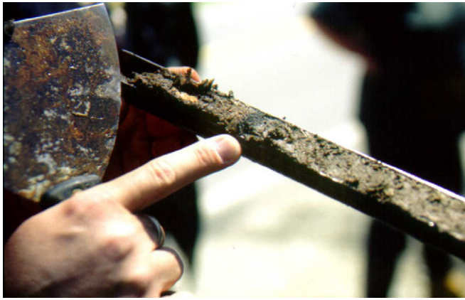
Figure 16. Photograph of paleotsunami deposit. Past tsunamis are recorded at Lagoon Creek in the parks. Tsunami deposits appear as sand layers in an accumulated organic-rich, peat-bog deposit. Lagoon Creek is a freshwater marsh protected from ocean waves by a beach berm, 6 m (20 ft) high. A tsunami would have to be robust and large enough to overtop this berm to deposit tsunami sand in the marsh. Dr. Gary Carver (Humboldt State University) extracted sediment cores from the Lagoon Creek in ca. 1996. NPS photograph courtesy of Vicki Ozaki (Redwood National and State Parks).
