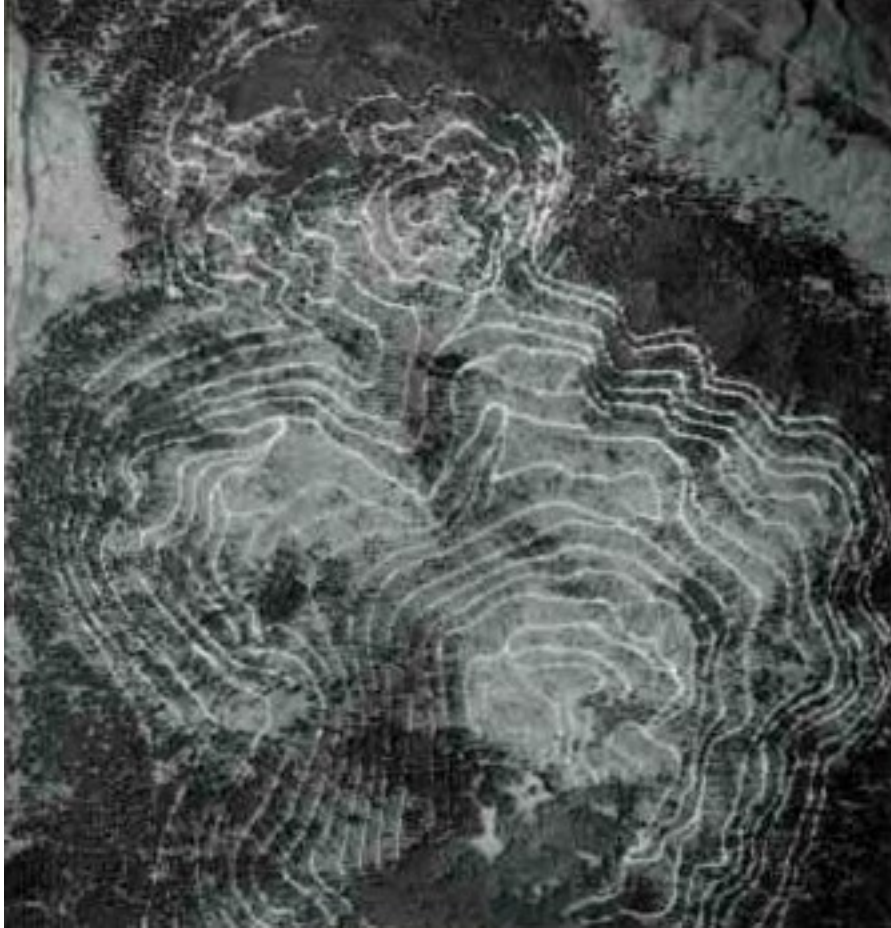
Figure 7.2. This aerial photograph, taken of Cerro del Abrigo in 1977, shows a network of logging roads that had been bulldozed out during the 1960s and early 1970s.
