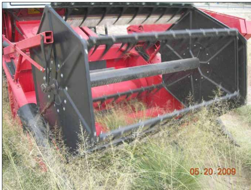
A close up of the front of the combine showing the cutter bars and tines. The tines help to move the cut materials through the combine's threshing tables.
