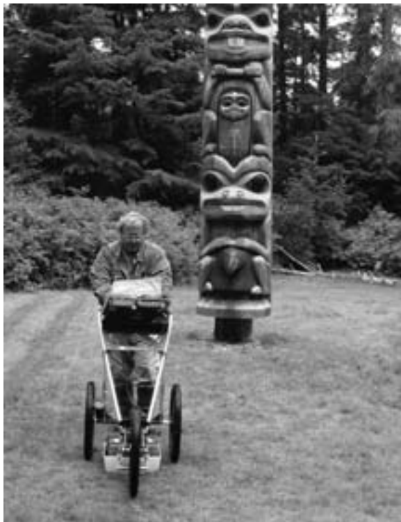
Figure 4-17. Ground penetrating radar (GPR) survey with cart system.
