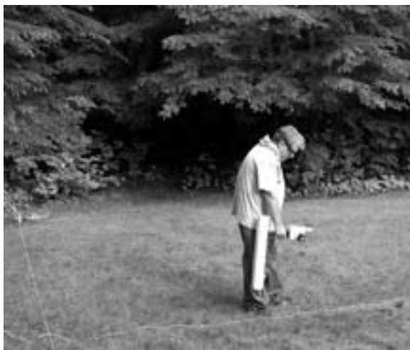
Figure 4-15. Magnetic gradient survey in the Fort Clearing using a fluxgate gradiometer.
