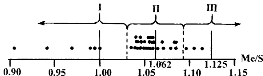
Fig. 3. Ratio Me/S in analyses of germanite. Groups of the analyses: (I) analyses with the relationship Me/S close to 1; (II) analyses with the relationship Me/S close to 1.062; and (III) analyses with the relationship Me/S close to 1.125.
