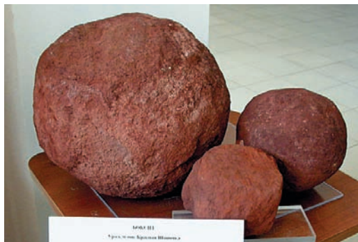
Photo 1. Bauxite. The Krasnaya Shapochka deposit, Urals. The size of the biggest sphere is 33 cm in diameter. VIMS Geological Museum. No 204sh. Photo: N.N. Krivoschekov.
