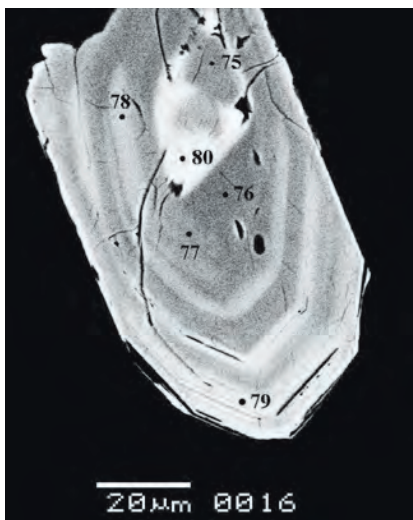
Fig. 11. Back-scattered electron image of aggregate pseudomorph of long-prismatic crystals of rutile after deformed and partly brecciated large plate crystal of ilmenite. The most deformed places are dissolved; pockets of crystals of monazite (white) are developed instead of them. Groundmass is composed of intergrown magnesite (dark gray), quartz (gray), potassium feldspar, and micas. Long fluorapatite (light gray) is above lamella.
