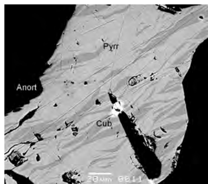
Fig. 1. Individual of pyrrhotite (Pyrr) consisting of two similar chemical varieties (light areas correspond to the enriched in iron), with ingrowths of cubanite (Cub) in anorthoclase matrix (Anorth), Kukisvumchorr Mt. (BSE-image).
