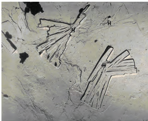
Fig. 2. Radiated segregations of uranophane-beta with nasturan (N) located in the cores of these segregations, Gornyi deposit, Central Transbaikalia. \times 7500 .
