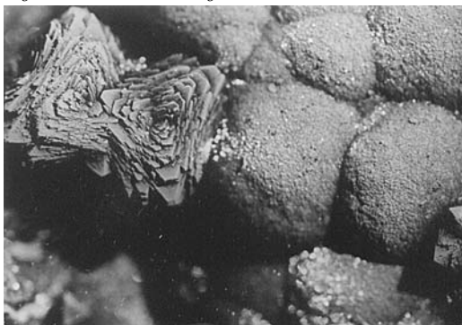
FIG. 3. Skeletal forms of block-crystals of pyrite of an octahedral habitus on a spherocrystalline crust of a siderite electronic microscopy-IMAGE in the dissipated electrons. A rib of an octahedron of ~1.2 mm
