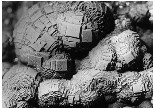
FIG. 5. Transition of a split cubooctahedron of pyrite into a spherocrystal: antiskeletal forms → initial phase of sphere formation. Photo of a sample sprayed-on with magnesium oxide on device FMN-2 (LOMO). Magnification x10
