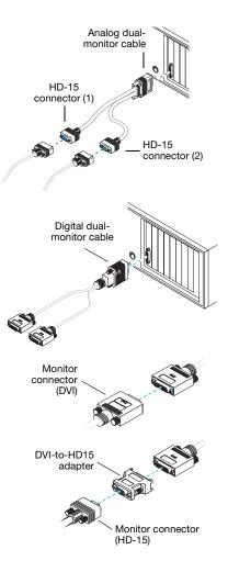
**Note:** Whenever you change your connection setup, make sure you're using the correct connectors and that all connectors are properly fastened.
