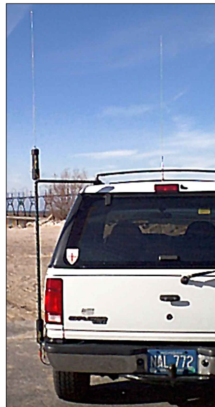
Ready for the road! A length of \frac{1}{2} -inch-diameter PVC pipe fastened to the vehicle's roof rack and antenna acts as a stabilizer.
