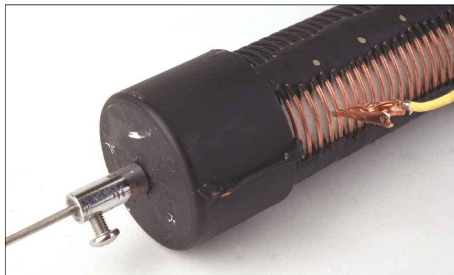
The loading coil resembles the matching coil except it has a greater number of turns. A RadioShack whip is attached to the top PVC cap. The wire lead connecting the bottom of the whip to the top of the loading coil passes through a hole in the top of the pipe cap.
