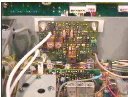
Figure 2—My IFD board installed in a Yaesu FT-736.
