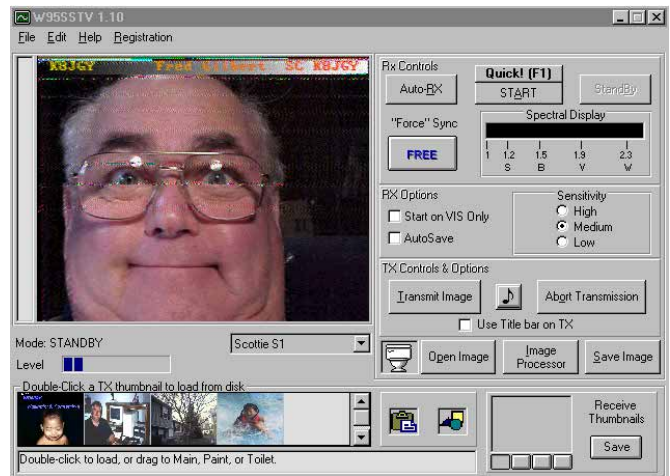
A happy K8JGY, as received on 20 meters (14.230 MHz). Noise appears as speckled horizontal lines.
