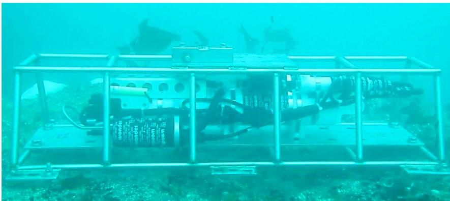
Figure 4. BOP housing a Seabird Electronics 16 Plus CT that measures temperature, conductivity, dissolved oxygen, and fluorescence.
