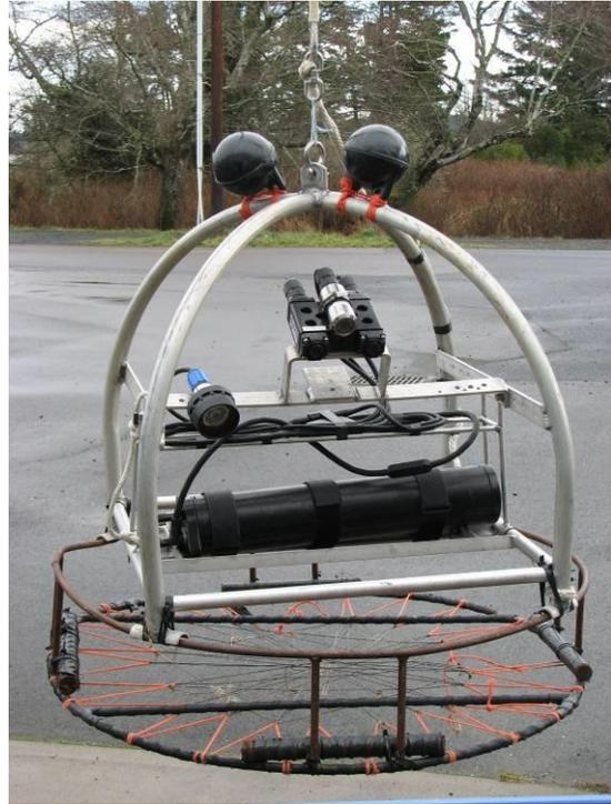
Figure 5. Video lander suspended by buoy line. At top is the breakaway link; at bottom is the breakaway base. Camera, lasers, light and pressure tube are mounted within the aluminum frame.
