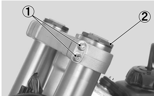
(1) UPPER PINCH BOLTS (2) FORK DAMPER
