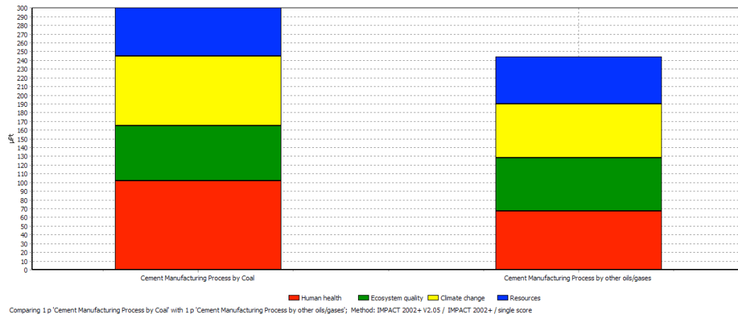
Fig. (7) The damage assessment of the two Egyptian cement plants (Endpoint Method)
