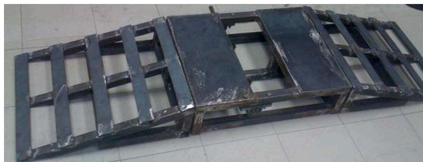
(a) Construction of RPG prototype
