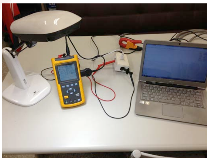
Fig. 3. Measurement circuit by Fluke 43B
