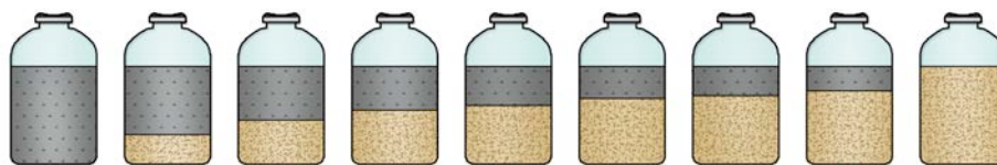
Fig. 1 Experimental batch serum bottle design
