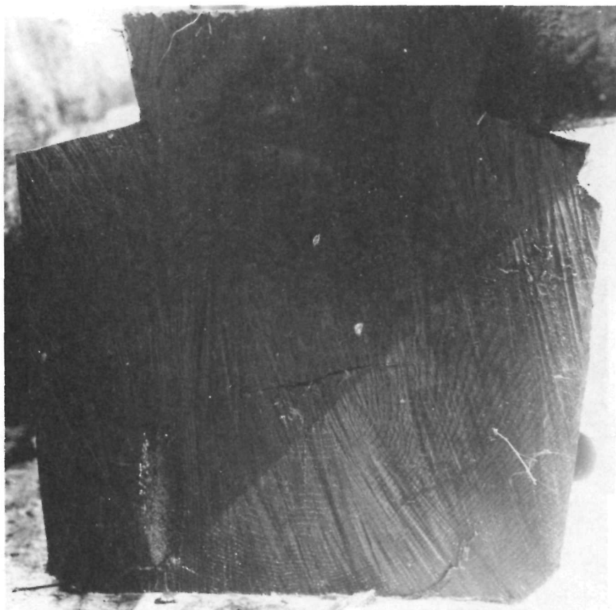
25 Cross-section of the stern keel cut. The keel is 14 inches in height. The orientation of the garboard rabbet is almost vertical.
