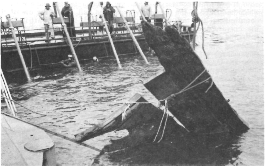
22 Rope sling around the stem-keel scarp of the stem-gripe assembly. Stopwaters in the scarp are still in place.
