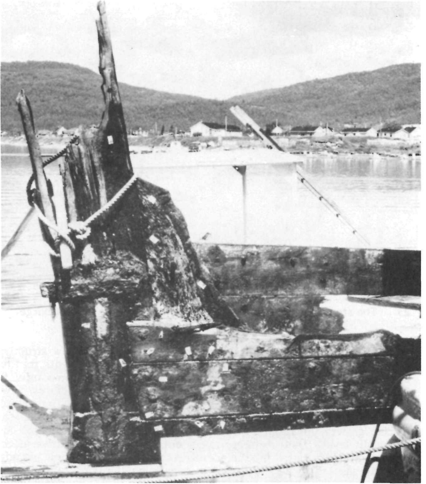
24 The heel of the Machault . The heel strap abutting the lowest gudgeon reinforced the mortise and tenon of the keel and sternpost.
