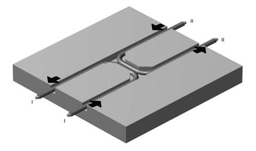
The following figure shows the routing of the TLS line cable for an inversion point:
