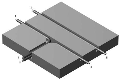
The following figure shows the routing of the TLS line cable for a two-way supply connection on the inside:
