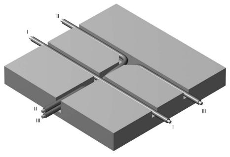
The following figure shows the routing of the TLS line cable for a two-way supply connection on the outside:
