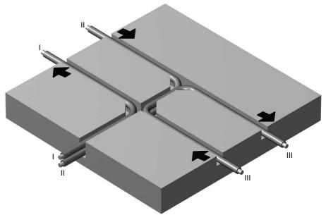
The following figure shows the routing of the TLS line cable for a one-way supply connection:
