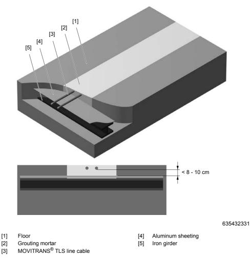
The aluminum sheeting must be at least 3 mm thick and should lie flush against the ferromagnetic material.
