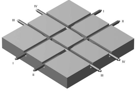
The following figure shows the routing of the TLS line cable for a crossing I (crossing tracks):
