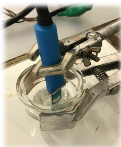
Figure 15. Electrochemical detection. Immersion of the SPAuE in K 4 [Fe(CN) 6 ]-3H 2 O in PBS 1X.
