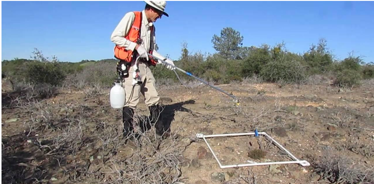
Figure 26. Phosphite application to marked seedlings at the 12.4kg/ha - 300 L/ha volume using a modified garden sprayer. The frame was placed over the seedling (visible near flag) and was marked to allow the applicator to time movement of the sprayer nozzle to an audio pulse generated by a metronome. White vinyl square with numbered tree tag is visible near the base of the seedling.
