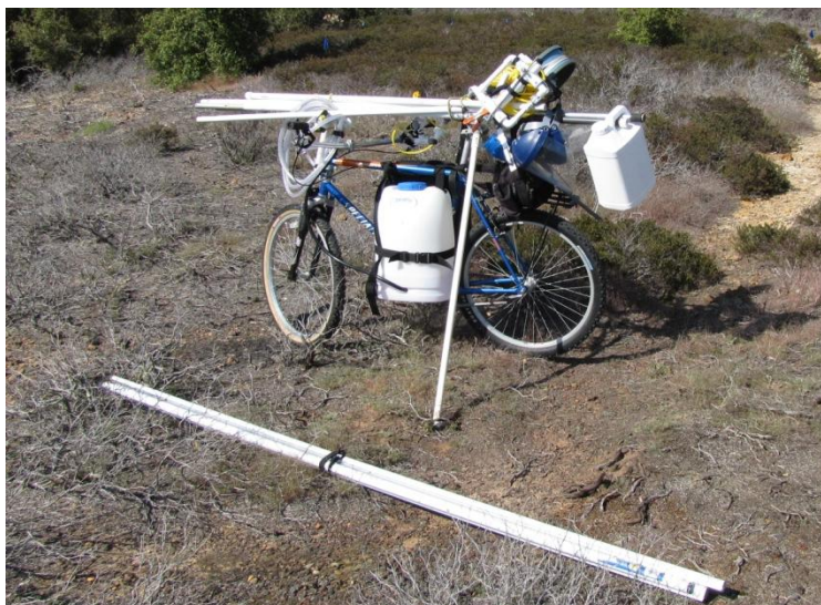
Figure 3. Spraying apparatus disassembled and packed for transport between plot areas. The entire apparatus is assembled and disassembled by hand by sliding sections together. Most joints are held together through the use of spring-action buttons. Four Phillips-head screws are used to lock two stiffeners in place.
