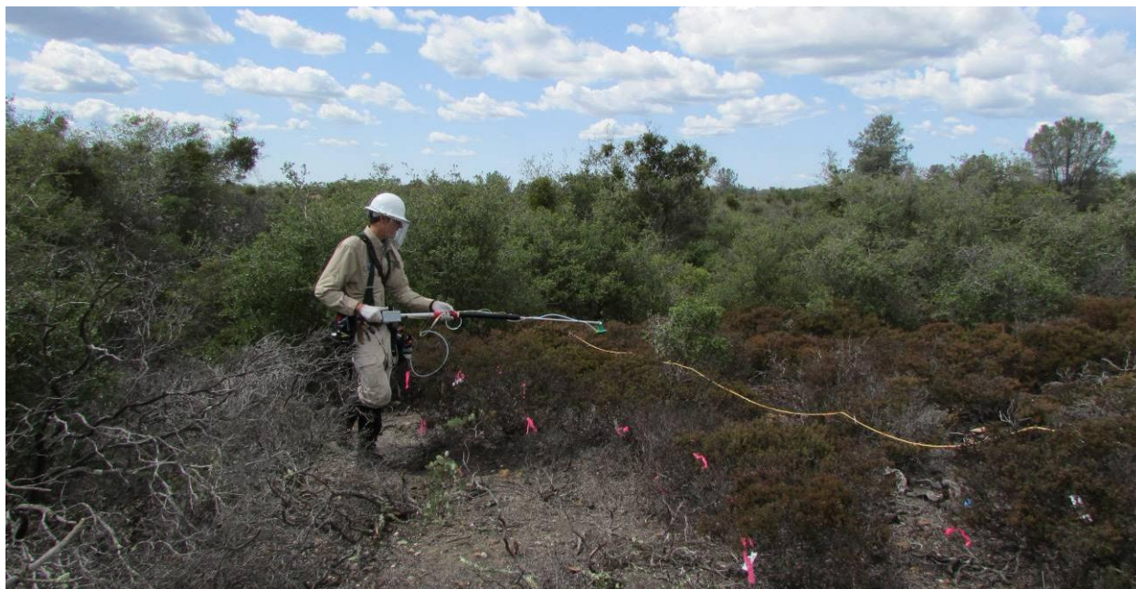
Figure 13. Spray being applied with CDA sprayer to plot 9W. The marked yellow rope was used as a guide to keep spray head velocity at the desired speed. The rope was marked at 0.25 m increments. The applicator moved the spray head across the plot using an audible beat from a metronome to time movement (1 beat per increment).
