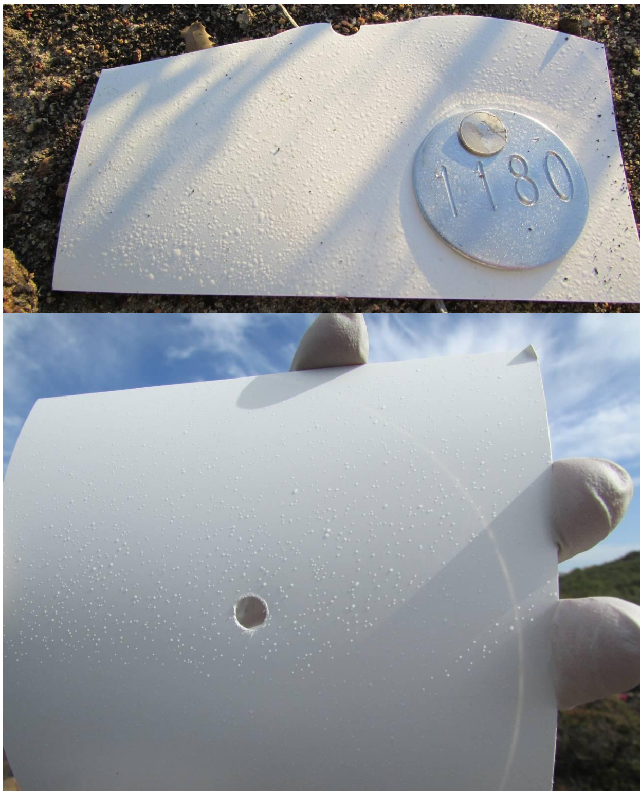
Figure 12. Top - 300 L/ha phosphite spray deposition on vinyl marker using the handheld sprayer shown in Figure 26. Bottom - 30 L/ha (ULV) spray droplet distribution on vinyl placed in a phytotoxicity trial microplot sprayed with the CDA sprayer.
