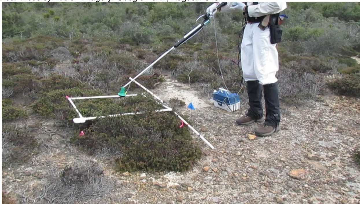
Figure 11. Application of potassium phosphite to microplot with the CDA sprayer. The PVC pole along one edge of the frame is marked in 24 cm increments. IPOD metronome was set so the audible signal prompted the applicator to move the spray head at the appropriate rate. Pink flags mark the corners of the microplot.
