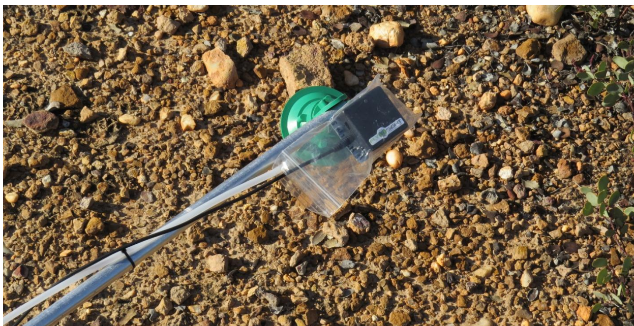
Figure 14. Head of the CDA with attached FlySight GPS unit. The FlySight is mounted on a metal plate that is magnetically attached to bracket on the spray head. The audio cable (black cord) runs back to portable mini speaker that is attached to the spray handle. The unit is placed in a plastic bag to protect it from blown spray.
