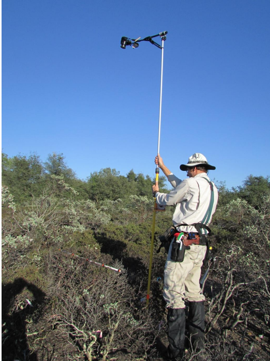
Figure 17. Overhead photo monitoring using camera mounted on an extendable pole. An angle gauge (partly visible below left forearm) was used to adjust the vertical angle of the pole. A 1 m reference stick (laying on top of the plants) is visible to left of camera pole.
