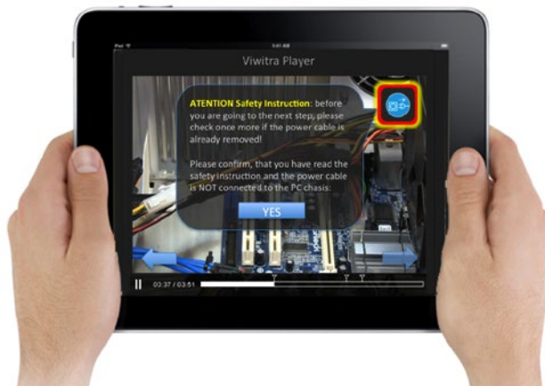
Fig. 6: Draft of the VIWITRA player with the danger information and confirmation functionality for removing the power cable
