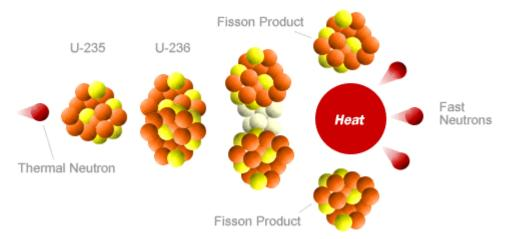
During fission the uranium atom splits into two roughly equal parts, known as 'fission products'. Spare neutrons are also released, along with heat from the energy holding the atom together. In isolation this process isn't very helpful as the heat released is very small and the spare neutrons move too quickly to be useful.
