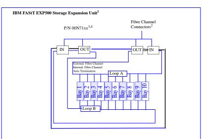
1. Housed in a 19" Rack mountable drawer and ships standard with redundant power supplies and two standard country power cables requiring separate power sources. Requires IBM industry standard 19" rack, EIA-310D, with a minimum depth of 24" (711.2 mm) or NetBAY3/3E.
