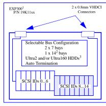
1. Housed in a 19" rack mountable drawer and ships standard with redundant 500 W hot-swap power supplies, two power cords and a single 2M Ultra2 SCSI cable capable of supporting Ultra160
