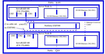
1.Customer supplied Ethernet Crossover Cable may vary in length up to a maximum of 25 feet (7.6 m).
