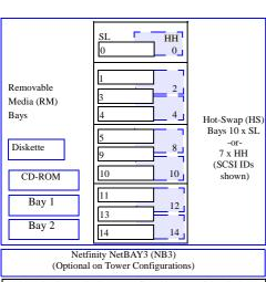
The top bay is HH; all others are configured in groups of three SL bays. When a HH drive is installed in one of these groups, only another HH or a single SL drive can be installed in the same group. For clarity, the SCSI IDs are identified.
