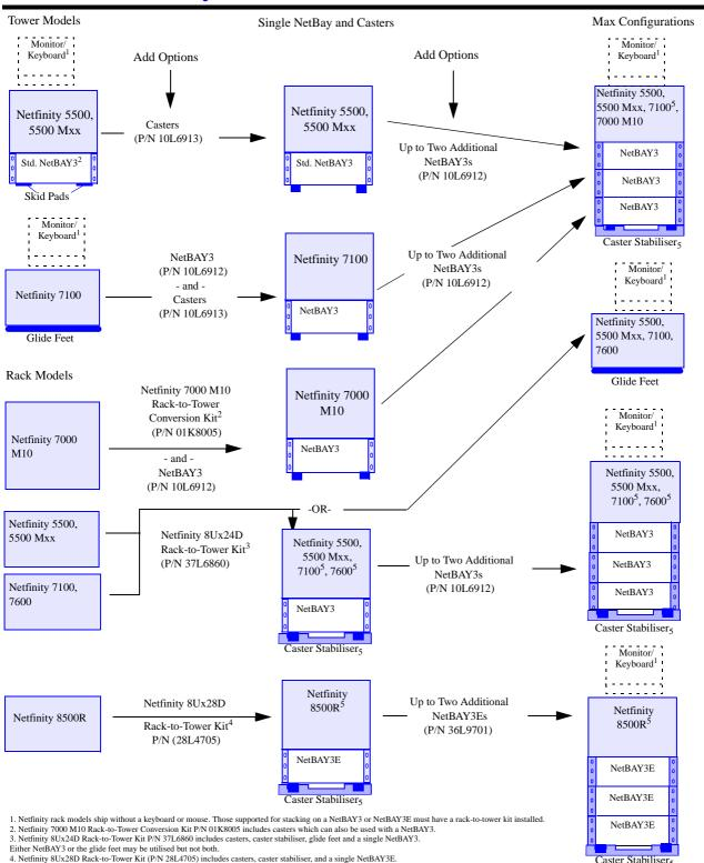
5. Netfinity 7100, 7600 and 8500R are not supported for installation with three empty NetBAY enclosures without a caster stabiliser. The caster stabiliser is included in Rack-to-Tower Kits P/N 37L6860 and P/N 28L4705 and is recommended for use with any quantity of NetBAY enclosures.
