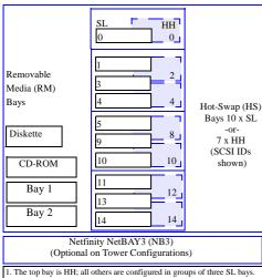
When a HH drive is installed in one of these groups, only another HH or a single SL drive can be installed in the same group. For clarity, the SCSI IDs are identified.
