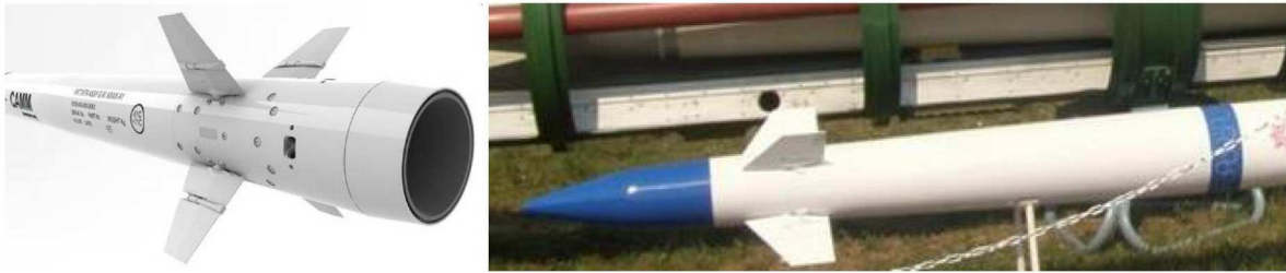
Rys. 1. (a) Lateral thrusters mounted on the CAMM [6], (b) mockup of a 9M96E missile with lateral thrusters installed
