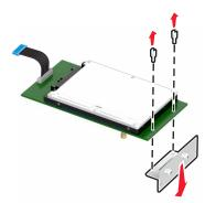
**b** Align the standoffs of the hard disk to the holes in the ISP, and then press the hard disk down until the standoffs are in place.
