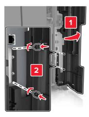
**c** Insert the plug of the hard disk interface cable into the receptacle of the controller board.
