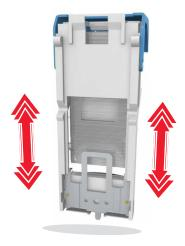
**7** Push the cartridge holder into the finisher until the holder *clicks* into place.
