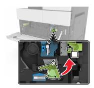
**4** Remove the photoconductor unit.
