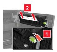
$\boldsymbol{3}\,$  Open the standard trays, and then locate the jammed paper.
