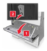
**2** Open door C. Make sure that it does not hit any cable attached to the printer.
