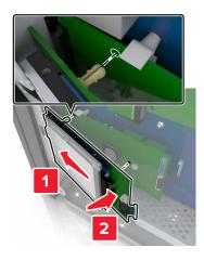
**c** Insert the plug of the hard disk interface cable into the receptacle of the ISP.
