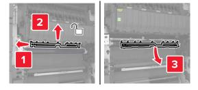
Lift the transfer module using the handles, and then pull it out completely.
