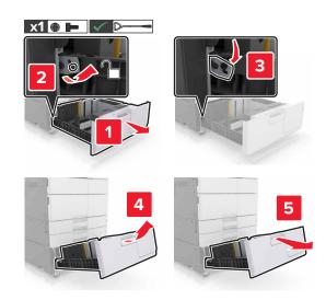
**3** Open door C. Make sure that it does not hit any cable attached to the printer.
