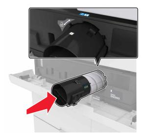
**5** Rotate the cartridge clockwise to lock it into place.
