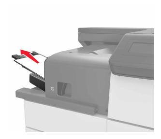
**2** Press the latch and slide the staple finisher to the left, and then remove the jammed paper.
