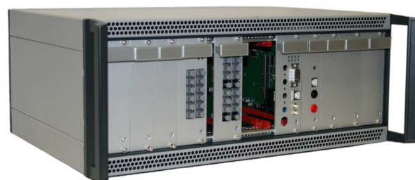
(h) control rack of Inverter 3
