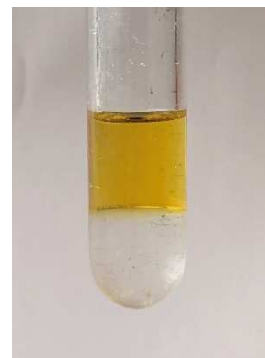
Figure 2. Observed partitioning of the Ru-MACHO-C 12 complex (53.90 mg) in a liquid–liquid biphasic mixture comprising n -decane (top, 2 mL) and an equimolar mixture of methanol and water (bottom, 1.42 mL/0.63 mL).
