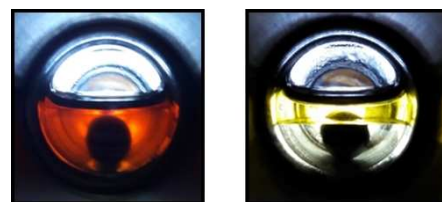
Figure 4. Observed reaction solution before (left) and after a typical hydrogenation experiment using dimethyl carbonate as substrate, where the spontaneously formed liquid product phase is clearly visible (right).
