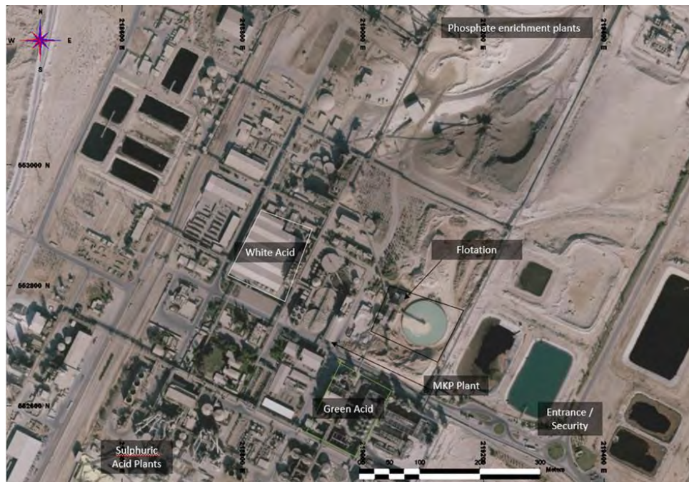
Figure 15.4: Rotem Process Plant Layout
