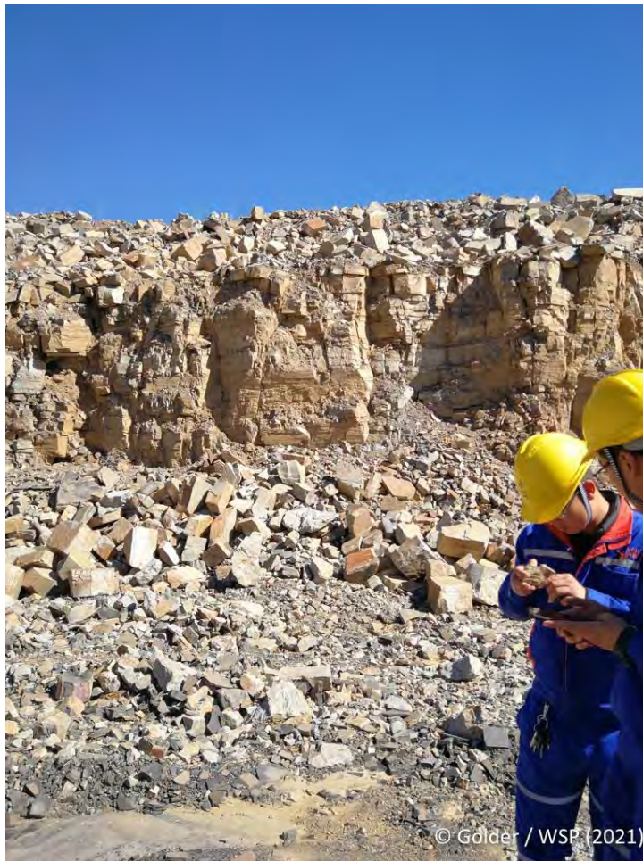
Photo 13.4: Upper Phosphate Layer Showing Fine Fragmentation from Blasting (Golder – November 2021)
