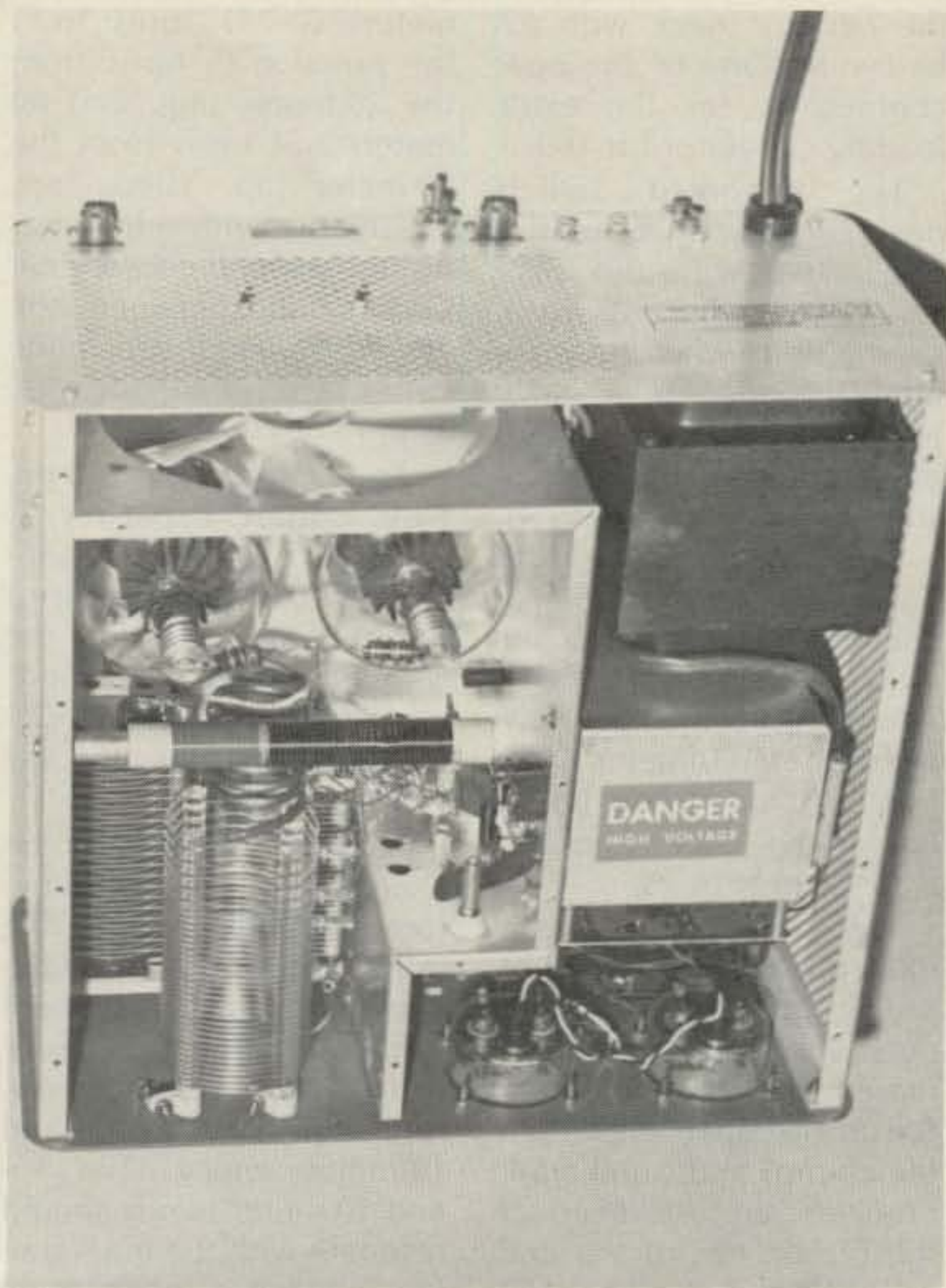
Photo B. The SB-221 converted for operation on 160 through 10 meters. The new tank coil is mounted on the front panel, using two holes that previously held a plastic Heathkit label. The new larger plate choke is mounted on the wall at left, using the original plate-choke standoff. The bandswitch is removed from the partition wall, modified, and replaced.
