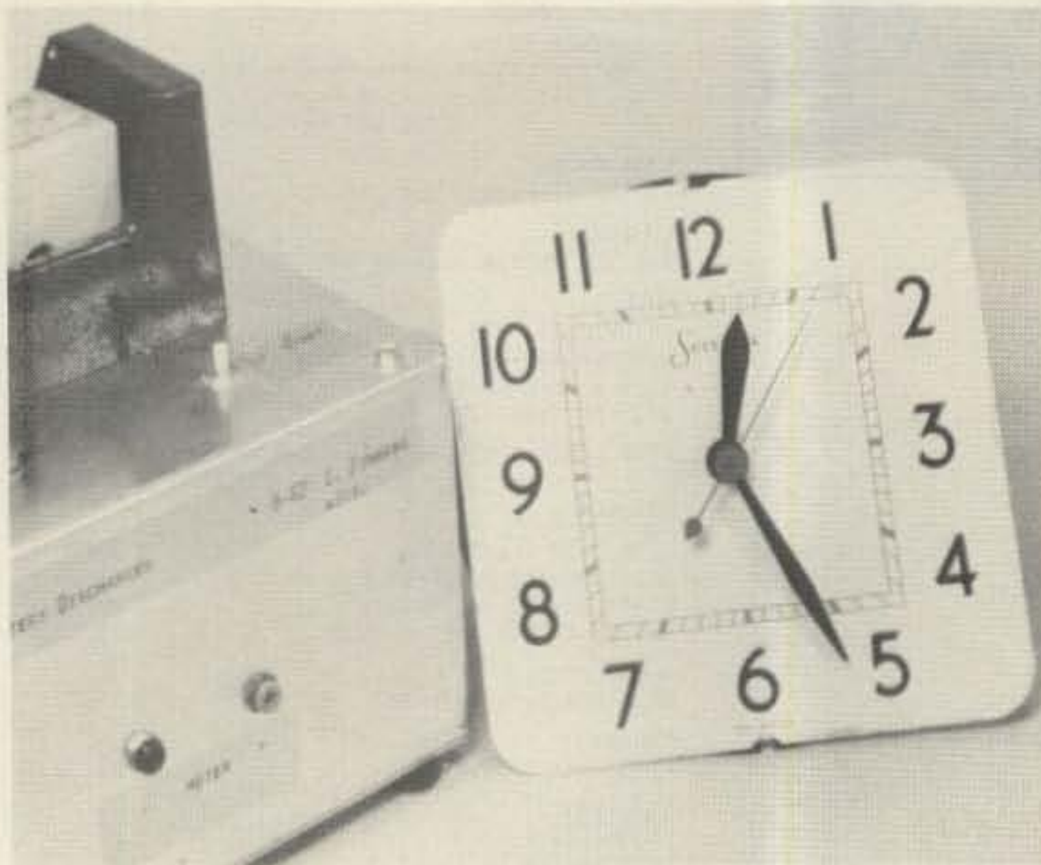
Photo D. If you don't like ICs, use an electric clock. This discharger uses the guts of an old kitchen clock as the timer.
