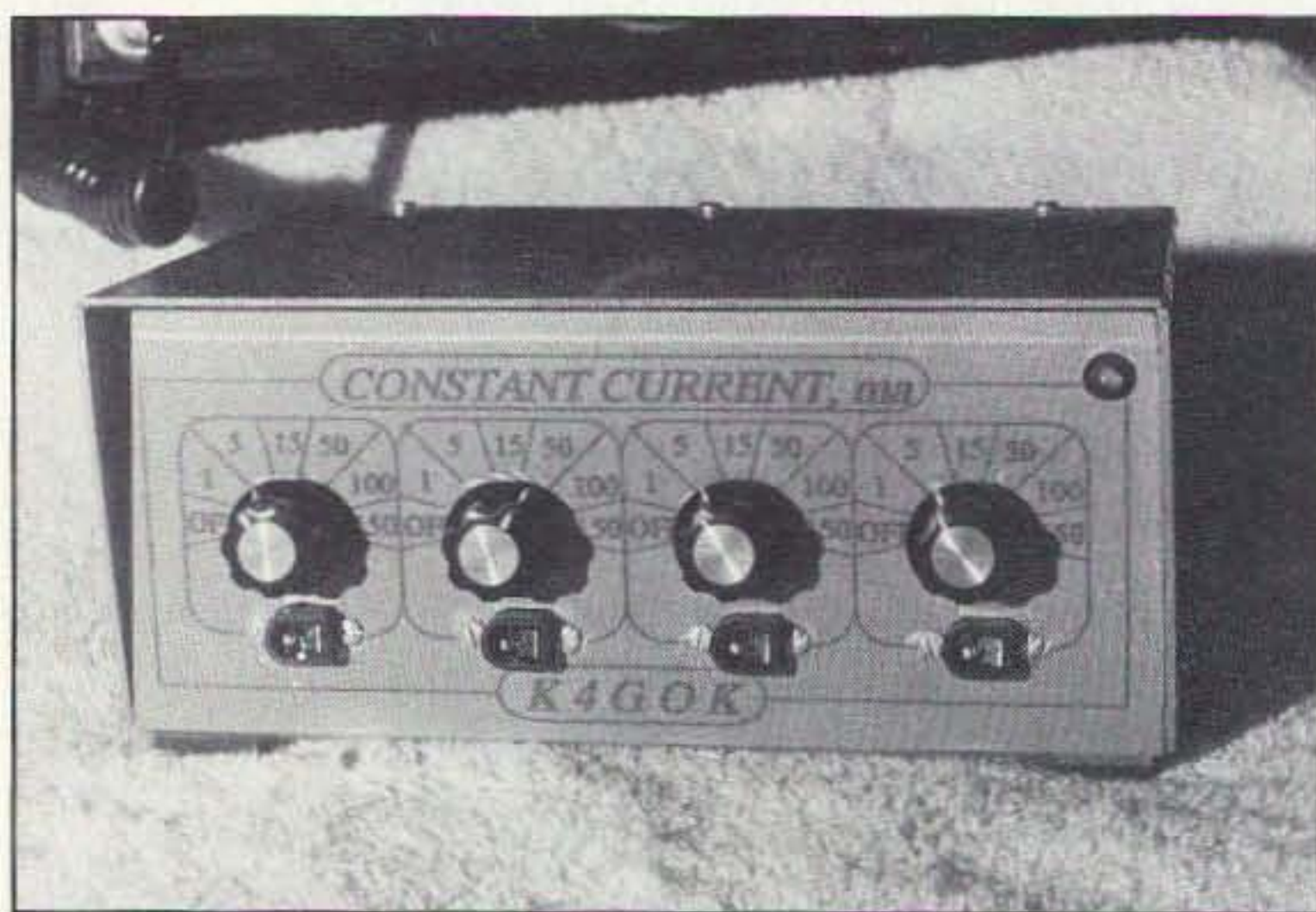
Photo A. The "CONSTANT CURRENT," panel made with a 9-pin dot matrix printer.
