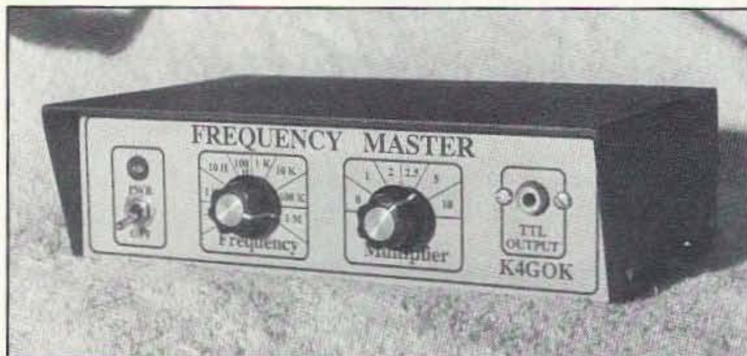
Photo B. Front panel of "FREQUENCY MASTER," showing the computer-generated panel layout.
