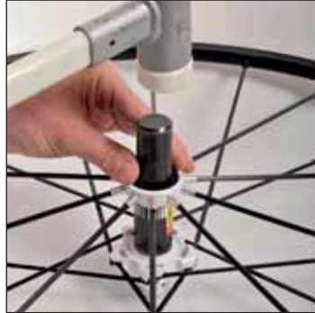
Fit the new bearings using bearing kit 323 909 01.
