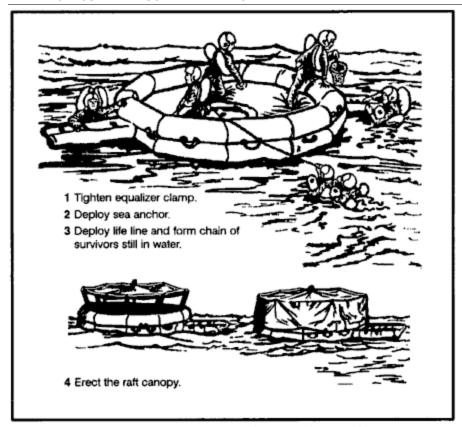
Figure 16-18. Immediate action-multiplace raft.
