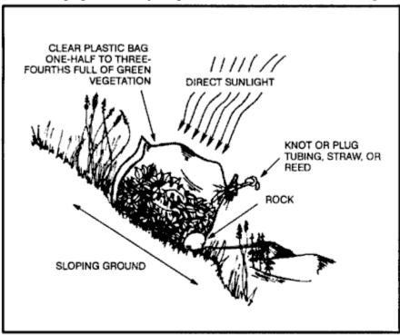
Figure 6-6. Aboveground solar water still.
