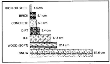
Figure 23-1. Thickness of materials to reduce gamma radiation.
