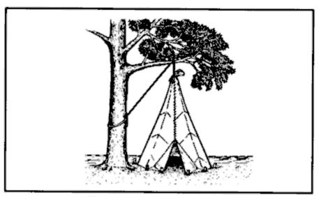
Figure 5-6. No-pole parachute tepee.
