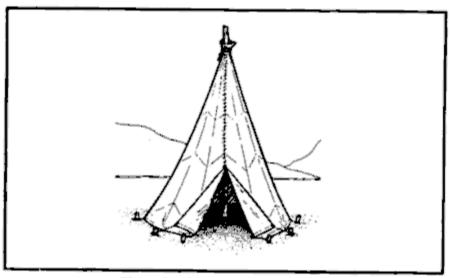
Figure 5-5. One-pole parachute tepee.
