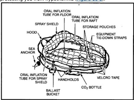
Figure 16-8. One-man raft with spray shield.
