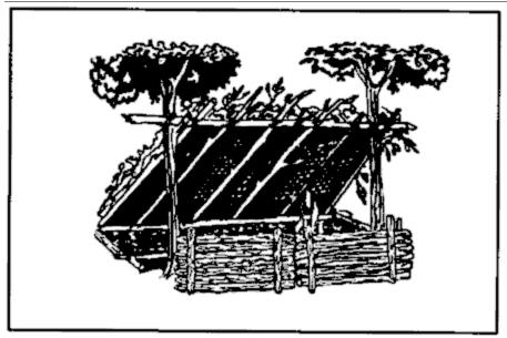
Figure 5-9. Field-expedient lean-to and fire reflector.
