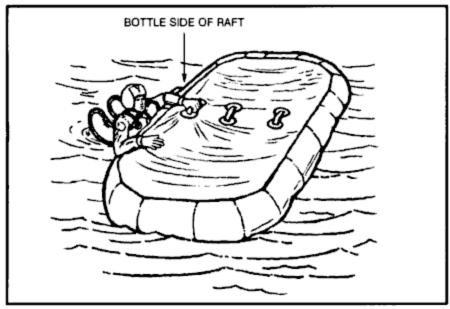
Figure 16-13. Method of righting raft.
