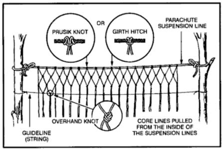
Figure 8-19. Making a gill net.
