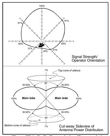
Figure III-1. Radio Transmission Characteristics
