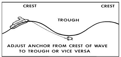
Figure II-11. Sea Anchor Deployment
