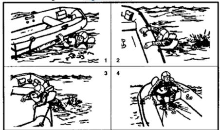
Figure 16-14. Method of boarding seven-man raft.
