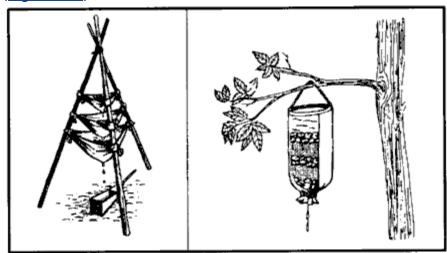
Figure 6-9. Water filtering systems.
