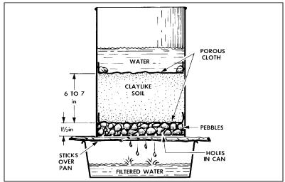
Figure IX-4. Filtration Systems, Filtering Water
