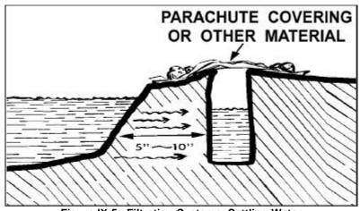
Figure IX-5. Filtration Systems, Settling Water
