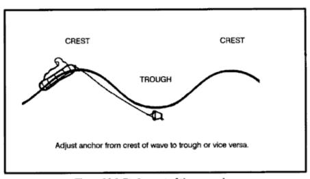
Figure 16-6. Deployment of the sea anchor.
