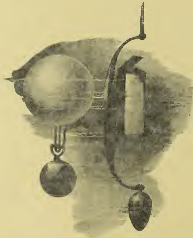
HOOKER'S SOUNDING MACHINE AND WATER-BOTTLE (see pp. 57 and 66)
