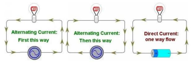
AC Sources: 1. Mains, 2. Output from Stabilizer, UPS and Inverter, 3. Generator etc
