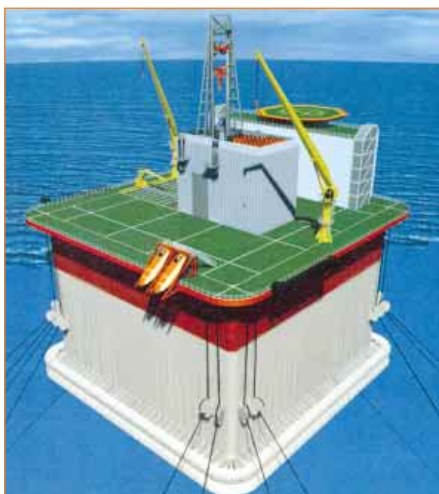
FOBOX (new design): Combining drilling and production capabilities with storage and offloading capabilities
