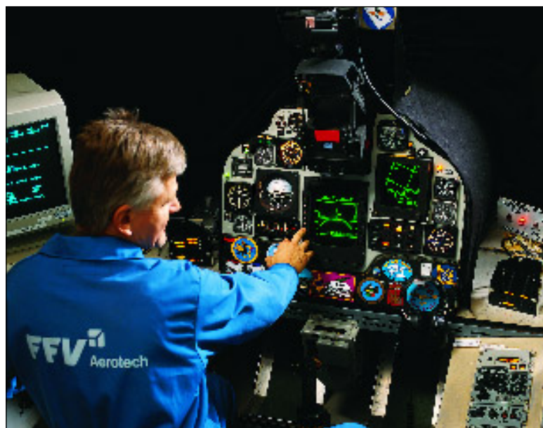
FFV Aerotech's JA 37 Test Rig is used for fault detection as well as testing software and installation modifications (right).
