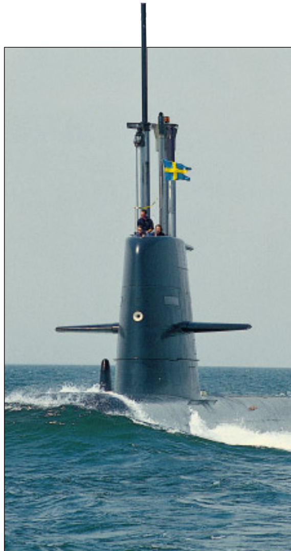
HMS Gotland, the Swedish Navy's new submarine, is the first series-built submarine in the world to feature an air-independent Stirling engine. The Stirling engine enables the submarine to stay submerged for long periods. The first in a series of three Gotland-class submarines, it was launched in February 1995.
