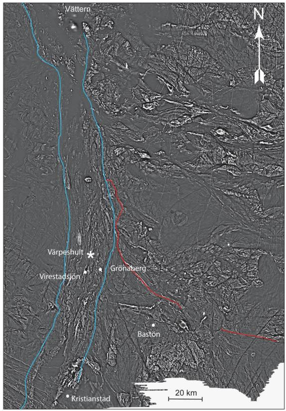
**Figure 3.** The magnetic field after filtering to enhance short-wavelength variations and thus enhancing the differences within the bedrock structures of the area. Locations as in figure 2. The Protogine Zone delimited by blue lines and the Blekinge-Bornholm province by red lines.
