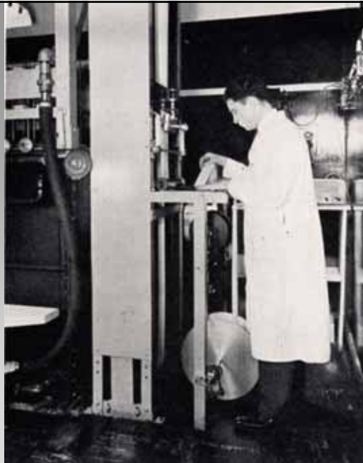
Pavelle Color laboratories, Feeding an exposed roll of Printon into processing system, 1950's. A Half Century of Color , Louis Walton Siple, 1951, page 158.
