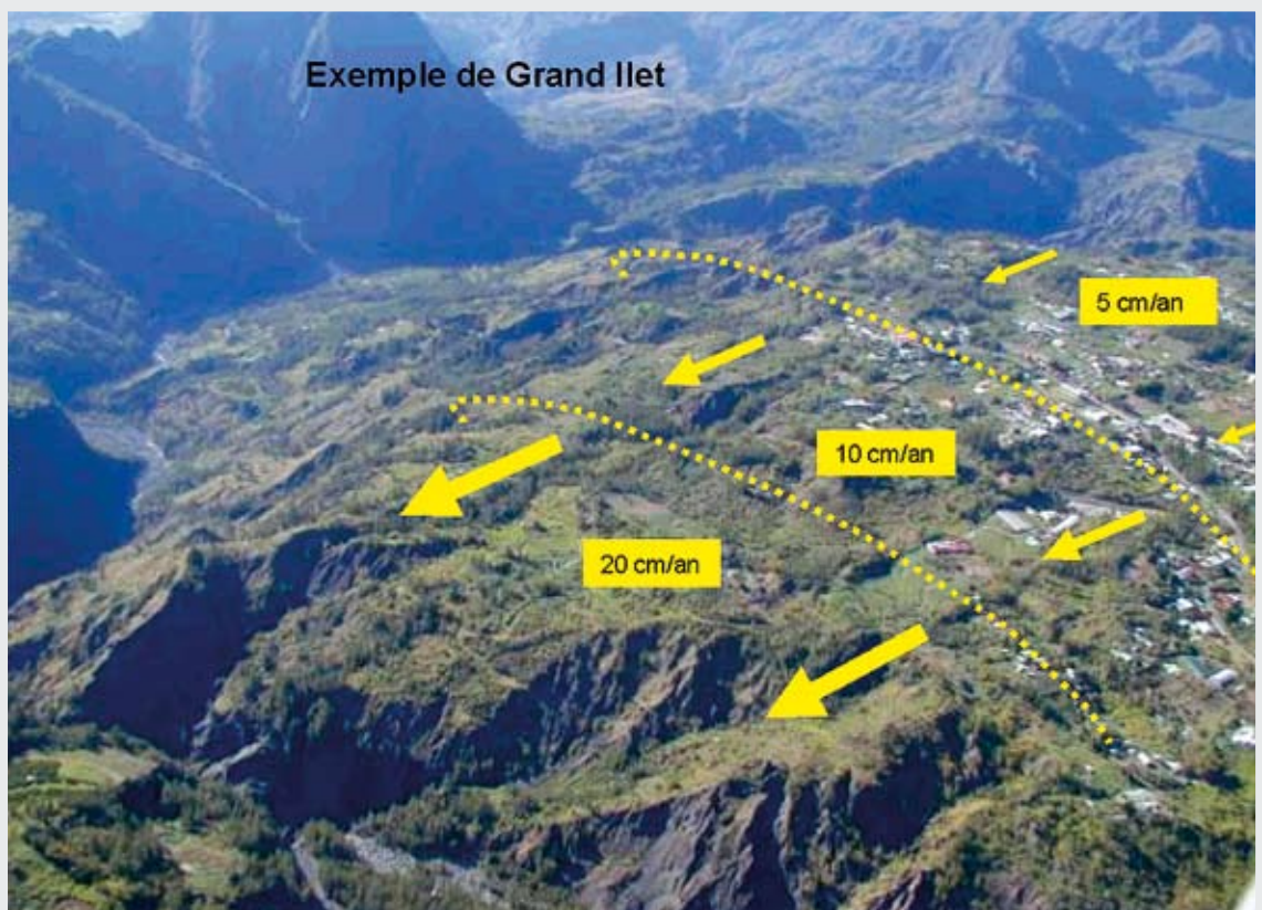
Figure 91 Glissement de terrain de Grand Ilet, cirque de Salazie (source: BRGM)
