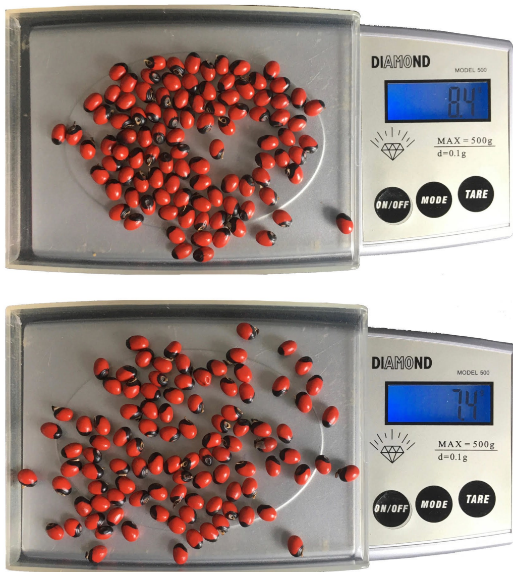
Weighing of 100 seeds of damma ( Abrus precatorius ) from Ivory Coast. Top, 100 heavy seeds, average weight 0.084 g (theoretical weight 0.083 g). Bottom, 100 light seeds, average weight 0.074 g (theoretical weight 0.073 g).
