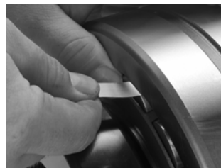
Fig. 14. Measure RIC before installation.
