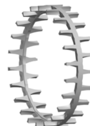
Fig. 8. One-piece, machined-brass, land-riding, finger-type cage.
