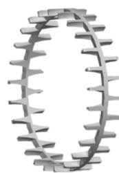
Fig. 7. One-piece, machined-brass, roller-riding, finger-type cage.
