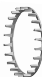
Fig. 9. Split, machined-brass, land-riding, finger-type cage.
