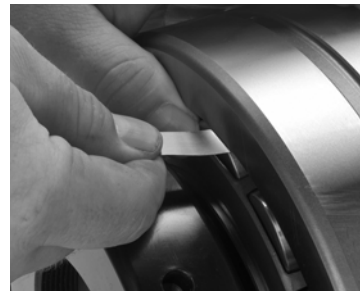
Fig. 18. Measure RIC before installation.
